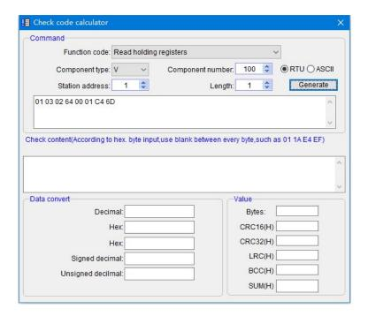
We choose the function code, set the type of components, component number, station number of slave PLC and so on, then click generate, you can get the command: 01 03 02 64 00 01 C4 6D, the command which sent by host computer can help to read the V100 value of PLC.
