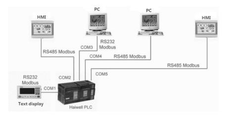
There is no need to write any program when PLC is used as slave, the default parameter is 19200 N 8 2 RTU, station number is 1. For configuration software and touch screen, which has the built-in Haiwell driver can directly select Haiwell driver, if there is no Haiwell driver, you can choose Modicon's Modbus driver. The corresponding Modbus communication code table of Haiwell is as the following figure:
