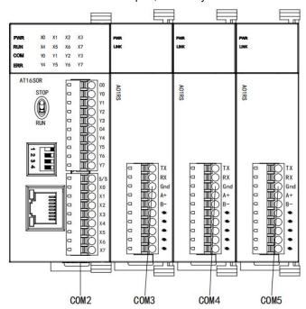
When the communication module is expanded, the communication port closest to the host PLC is COM3, next is COM4 and last is COM5. The position of communication module can be random, and the communication port number can be viewed in the hardware configuration, as shown in the figure below:
