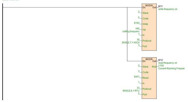
Port = 3, in this example, it indicates the communication port of S01RS. 8193 can be quickly entered, such as put the mouse on the "Write" terminal, then it can directly enter 0x2001.
