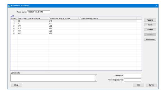
In the Haiwell PLC programming software, set up Haiwellbus write communication table, as follows:
