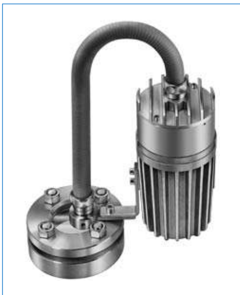
Fibre-optic lightpipe light fitting with built-in timer "U", type fibroLUX® W W2 U sp, EEx de IIC T3, Ex II 2 G + D, 50 W, 24 V DC, fixation of the light source by bracket "W", fixation of the lightpipe by universal support "W2" onto sightglass to DIN 28120, DN 40, PN 10
