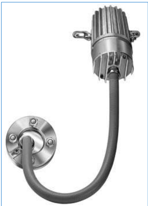
Fibre-optic lightpipe light fitting for use in hazardous areas with built-in timer "V", type fibroLUX® X1 W2 V, EEx de IIC T4, Ex II 2 G + D, 50 W, 230 V, fixation of the light source by fixation legs "X1", fixation of the lightpipe by universal support "W2" onto sightglass to DIN 28120, DN 40, PN 10
