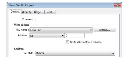
5. Add Set Bit objects on the [Enter] and [ESC] Function Key objects respectively. Set address to [LB-0] and [Set style] to [Set OFF]. In this way when pressing either [Enter] or [ESC] key will close the keyboard window.
