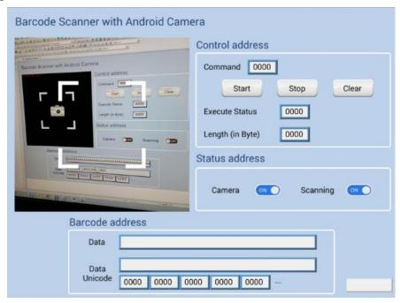
3. When a QR code is read, the Execute Status turns 1, and the QR code is captured, its content will be displayed in Barcode Address group box. Unicode is also supported.
