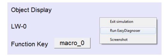
5. Afterwards, EasyDiagnoser will be started. [Logger] window displays whether EasyDiagnoser is able to connect with the HMI to be watched or not. [Output] window displays the output of the TRACE function. The illustration below shows that EasyDiagnoser succeeds in connecting with HMI.
