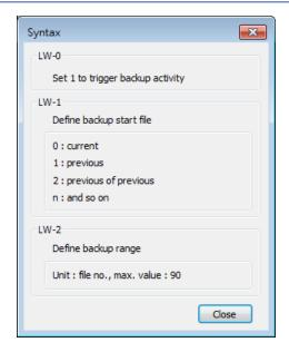
On cMT-SVR, Backup (Trigger-based) object only supports [Touch trigger] mode but not [External trigger (bit)] and [External trigger (word)] modes.
