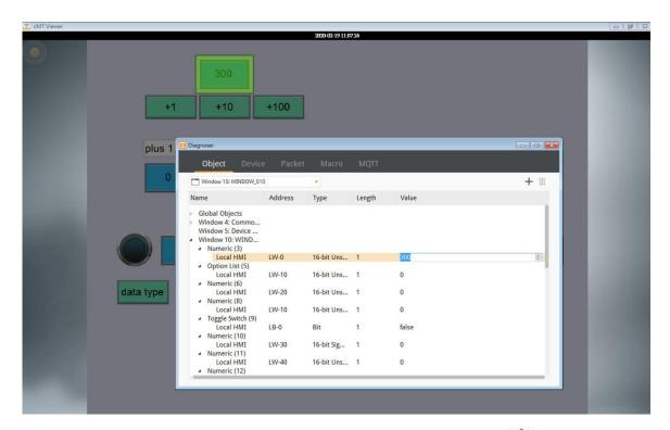
5. In cMT Diagnoser, watch addresses can be added or deleted. Click to add a new address, or select an address and then click to delete it.
