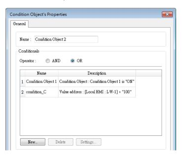
3. Now the Condition objects can do the same thing as the macro, which triggers actions according to the conditions.
