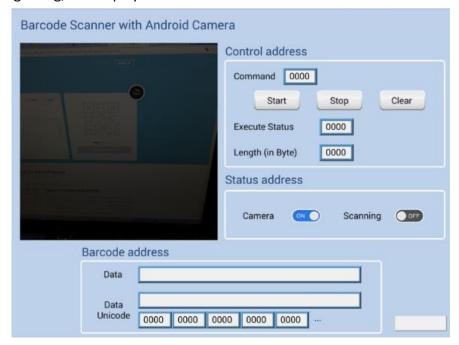
Tap Start button, the status of Scanning turns ON, the display turns bright, and is ready for scanning.
