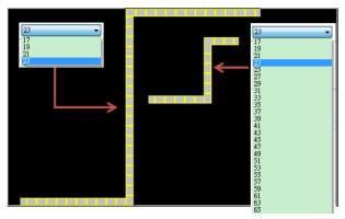
To prevent the flow block from overlapping itself, when the distance between two lines is shorter (Section A), the valid range is restricted. When the distance is longer (Section B), the adjustment range will be larger.
