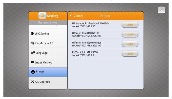
3. Select a network printer and tap [Install] to install its driver. The new printer driver will replace the former one since only one printer can be installed at a time.
