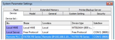
Device\_type is the device type and encoding method (binary or BCD) of the device data. For example, if device\_type is LW\_BIN, it means the register is LW and the encoding method is binary. If use BIN encoding method, "\_BIN" can be ignored.
