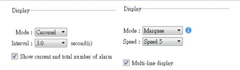
When [Carousel] mode is selected, the option to display the current and total alarm count and set the interval in seconds can be enabled.
