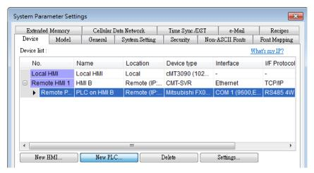
5. Create a Set Bit Object, select "PLC on HMI B" in [PLC name] to control the PLC connected with the remote HMI B.
