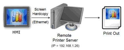
Users can make screen hardcopies with a Function Key object. The hardcopies will be transferred to the Remote Printer Server via Ethernet and then printed out.
