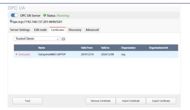
Note: According to OPC UA specification, an OPC UA client, in making a connection, will use a client certificate which will be checked by the OPC UA server for its legitimacy. The exception is if the security policy allows for the "None" option.
