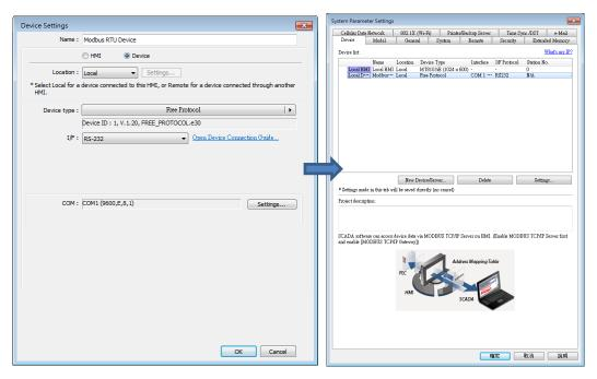
2. The interface of the device (I/F) uses [RS-232]. If a MODBUS TCP/IP device is connected, the interface should be [Ethernet] with correct IP and port number as follows:
