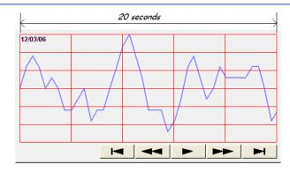
Select [Time] for [X axis time range] and go to [Trend] » [Grid] and enable [Time scale]. Please refer to [Time scale] in the later section.
