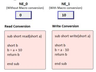
3. Enter 80 in NE\_1, [Write conversion] is executed and the value gained will be 70. NE\_0 displays 70.
