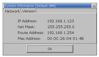
2. On PC, enter the HMI IP address: <a href="ftp://192.168.1.123">ftp://192.168.1.123</a> (example), then log in by the user name: uploadhis, and enter the HMI [history upload password] (if not changed, the default password is 111111). Or, directly enter <a href="ftp://uploadhis:111111@192.168.1.123/">ftp://uploadhis:111111@192.168.1.123/</a>
