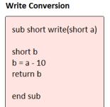
Create two Numeric objects: NE\_0 and NE\_1 and use the same control address. Select [Macro subroutine] for NE\_1.
