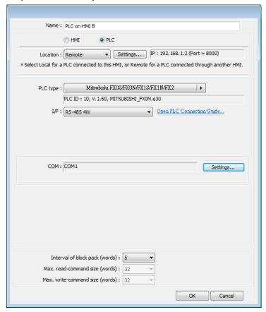
3. Create a Set Bit Object, select "PLC on HMI B" in [PLC name] to control the PLC connected with the remote HMI B.
