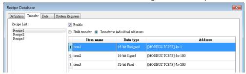
Under this mode, the data type setting of each destination addresses must also follow those of the corresponding recipe item. In the settings shown above, the data type of address 4x-1 should be 16-bit Signed, and 4x-100 should be 32-bit Signed, and so on.
