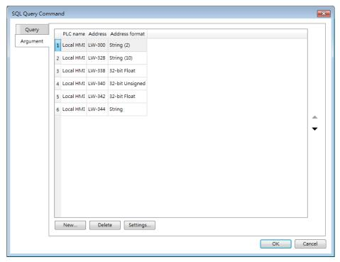
If argument is used in the syntax of a command in [Query] tab, the system will refer to the address specified in this tab according to the argument number enclosed in \${argument no.}.
