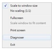
2. To permit connection to HMI from cMT Diagnoser, enable the Diagnoser option which is found in the [System Parameters] » [Remote] tab in EasyBuilder Pro.
