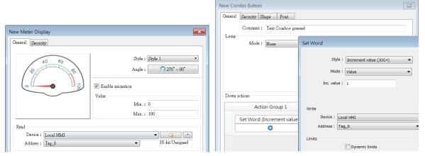
**4.** Set the Combo Button's comment to "Text Combo+ pressed" and its text label to "Combo+".
