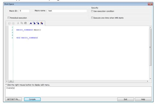
3. Design your macro. To use built-in functions (like SetData()) or GetData()), press [Get/Set FN...] button to open API dialog box and select the function and set essential parameters.
