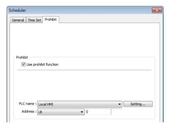
Before the scheduled action is performed, the HMI will read the specified bit state. If it is ON, the scheduled start/end action will be skipped. Otherwise, it will be performed normally.
