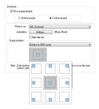
6. Select "200.Keyboard". When you press Numerical Input or ASCII Input objects on the screen, "window no. 200" will pop up. You can press the keys on the keyboard to enter data.
