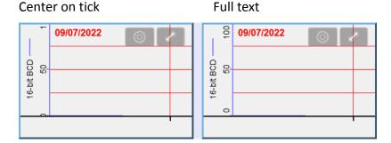
Y Scale can be configured on the in cMT Viewer as shown in the following steps.
