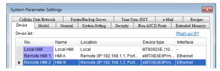
3. Create a Set Bit Object, select "HMI A" in [PLC name] to control the address of the remote HMI A. Same for the HMI B.
