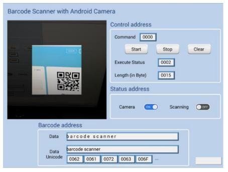
5. After changing to another page, Scanning turns OFF, the parameters are reserved. The parameters will be cleared when next time Start button is tapped, or Clear button is tapped.
