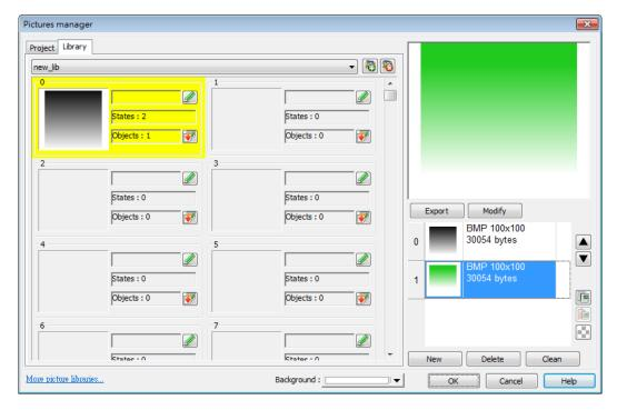
9. When finished, a complete Picture is created, click [OK]. In [Picture manager] dialog box it shows that the newly added Picture Number 0 is a bitmap picture with two states.
