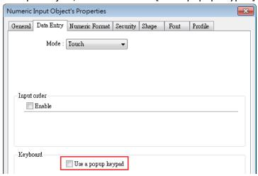
4. Create a Set Bit object, set address to [LB-0] and set [Set style] to [Set ON]. Overlay it on the Numeric Input object. Pressing the Numeric Input object will open the keyboard window.
