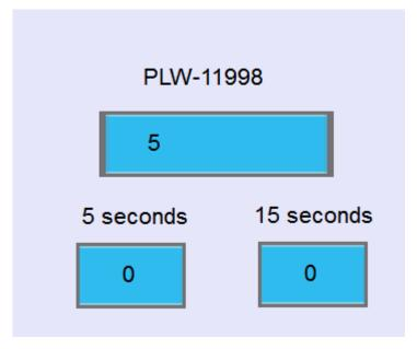
After 5 seconds, the bottom left object turns grey due to expired control token, and another object has 10 seconds left for countdown.
