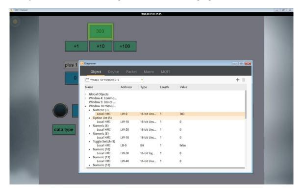
4. The value of an object can be changed by double-clicking on it in cMT Diagnoser window.
