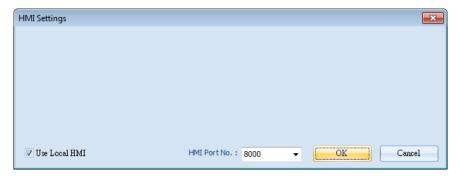
2. Select a target HMI or PLC. If one HMI is selected, you can directly control the local HMI.
