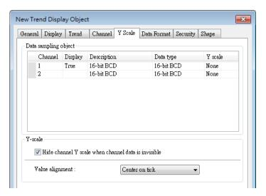
The scale along the Y axis of a specific channel can be displayed. To enable Y Scale, [Grid] should first be enabled in [Trend] tab.
