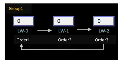
2. When finish entering data in the last object, to end data entry of all objects, please select [Stop sequential input function after input] check box.
