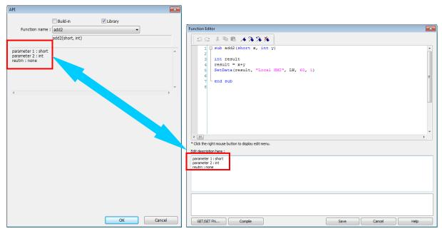
**5.** Select the function to be used, fill in the corresponding variables according to the data type.
