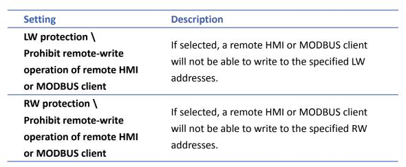
Click [Data Security] button to set the restrictions on the write operations that modify local Word or Bit register data.
