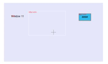
**4.** By entering a window number in the Numeric Input object, the Indirect Window is displayed according to the selected style.
