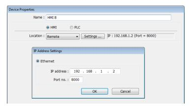
**3.** Create a Set Bit Object, select "HMI B" in [PLC name] to control the address of the remote HMI.
