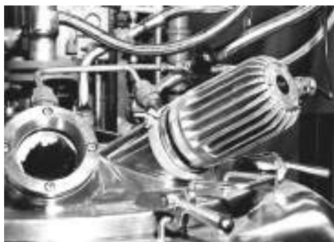
High performance sightglass light fitting type R 100 deHSch, 100 W, Ex d e IIC T3 Gb, Ex t IIIC T195°C Db IP67, Ex II 2 G + D, on a basket centrifuge
