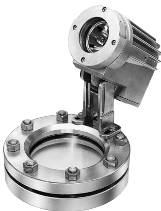
Type PEL 20 deH Sch, 230 V, 20 W, Ex d e IIC T6 Gb, Ex t IIIC T80°C Db IP67, Ex II 2 G + D, mounted on circular sightglass to DIN 28120, DN 125, PN 10, in 1 port version
