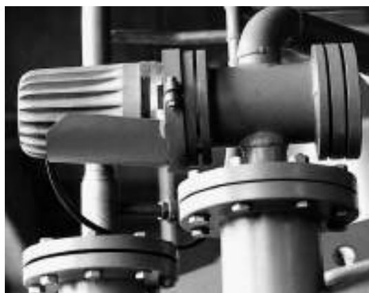
CHEMLUX ® sightglass light fitting, type L 20 deH M sp, 20 W, 24 V, Ex d e IIC T5 Gb, Ex t IIIC T95°C Db IP67, Ex II 2 G + D, mounted with an opal glass screen "M" on a pipeline flow indicator
